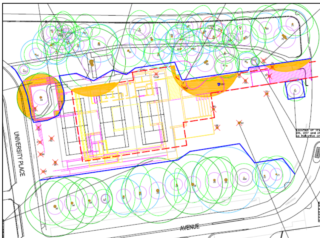
Figure 11: Excerpt from Tree Protection Plan (ASTPP01 Rev 2 03/05/2017) showing proposed building footprint in relation to site trees. Source: ArborSafe, May 2017
