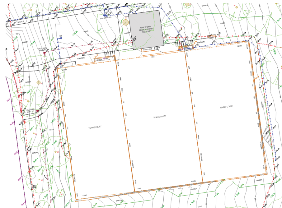
Figure 15 In-ground survey extract indicating existing underground cables within the site
