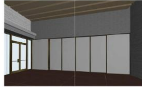
OPTION 3: OPENING: 4.8m(w) x 3.6m(h) EQUAL SIDE PANELS 4 EQUAL DOORS
