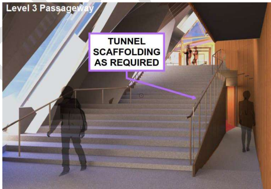
Figure 163- Access Tunnel Scaffold
