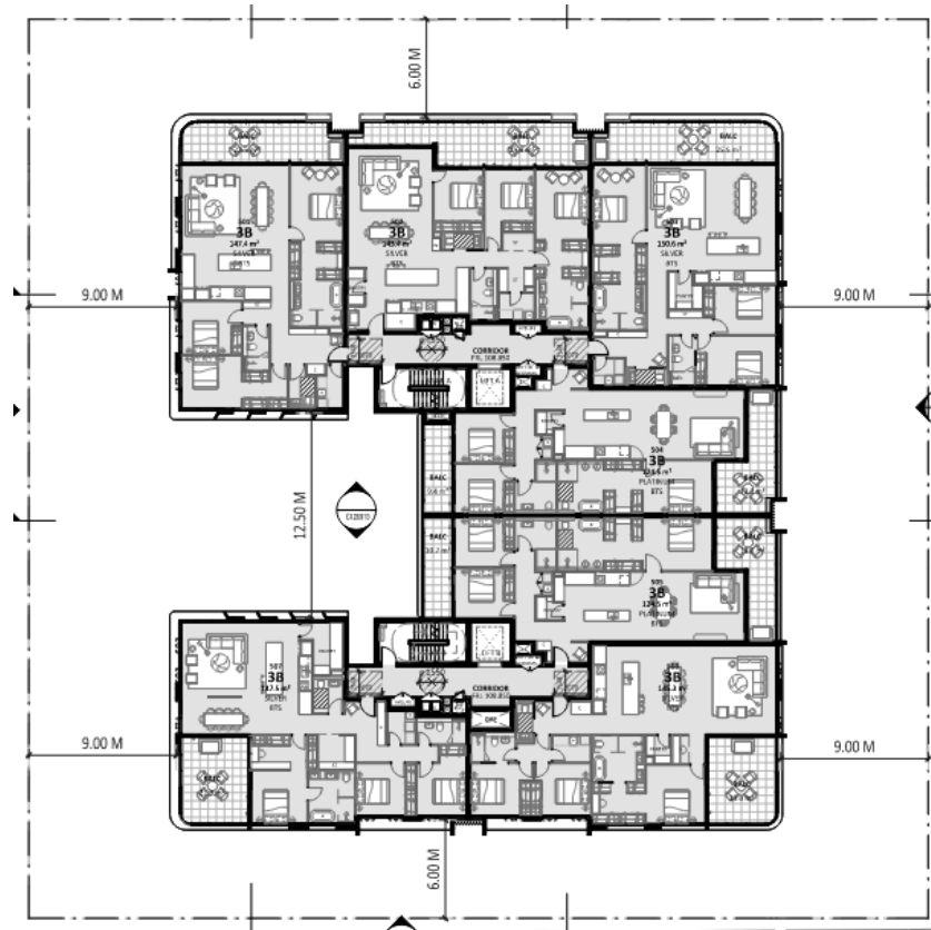
Figure 12 - General arrangement Level 06
