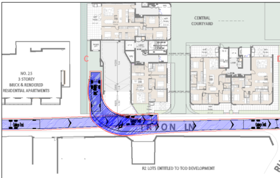
Figure 44 Swept paths - Loading Area (Source: JMT)
