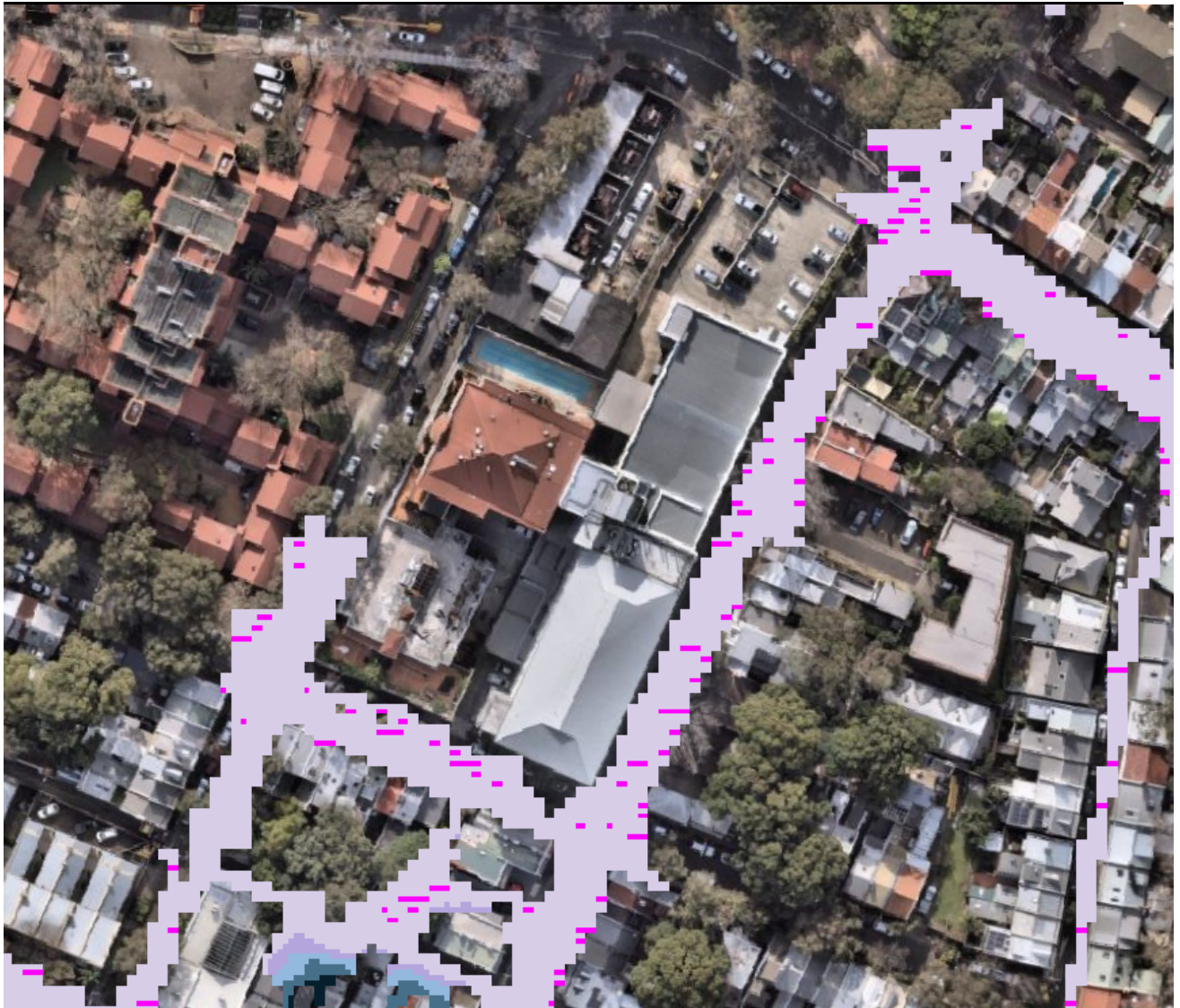
Figure 16 – Flooding Extent during 1% AEP Flood Event within the Vicinity of the Site (Source: Alexandria Canal Flood Model).
