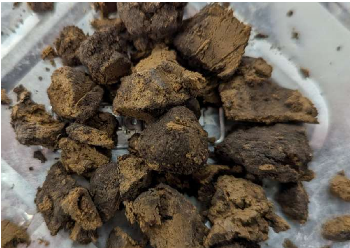
Photograph C6: Image of the S10 from 0.7 mbgl of BH7. Yellow-Brown Sandy Clayey Soil with trace rootlets observed inside.
