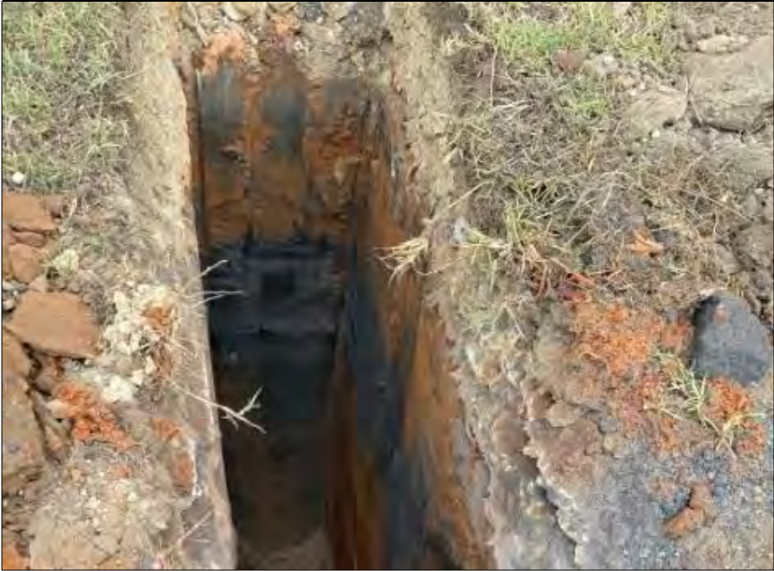
PHOTO 7: 'FLY ASH' EXCAVATED FROM P_TP07 AT 0.4-0.7 M BGS
