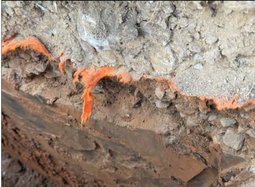
PHOTO 12: LAYER OF GEOFABRIC AT P_TP04 FROM 0.3 M BGS
