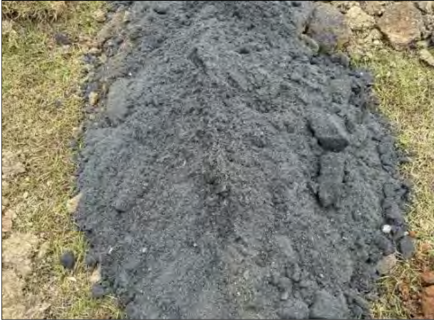
PHOTO 7: 'FLY ASH' EXCAVATED FROM P_TP07 AT 0.4-0.7 M BGS
