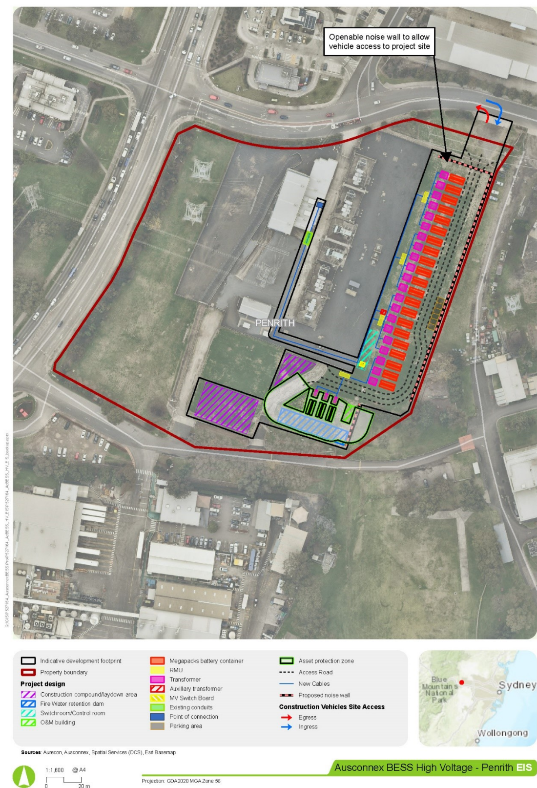
Figure 1-3: Penrith HV BESS general arrangement layout
