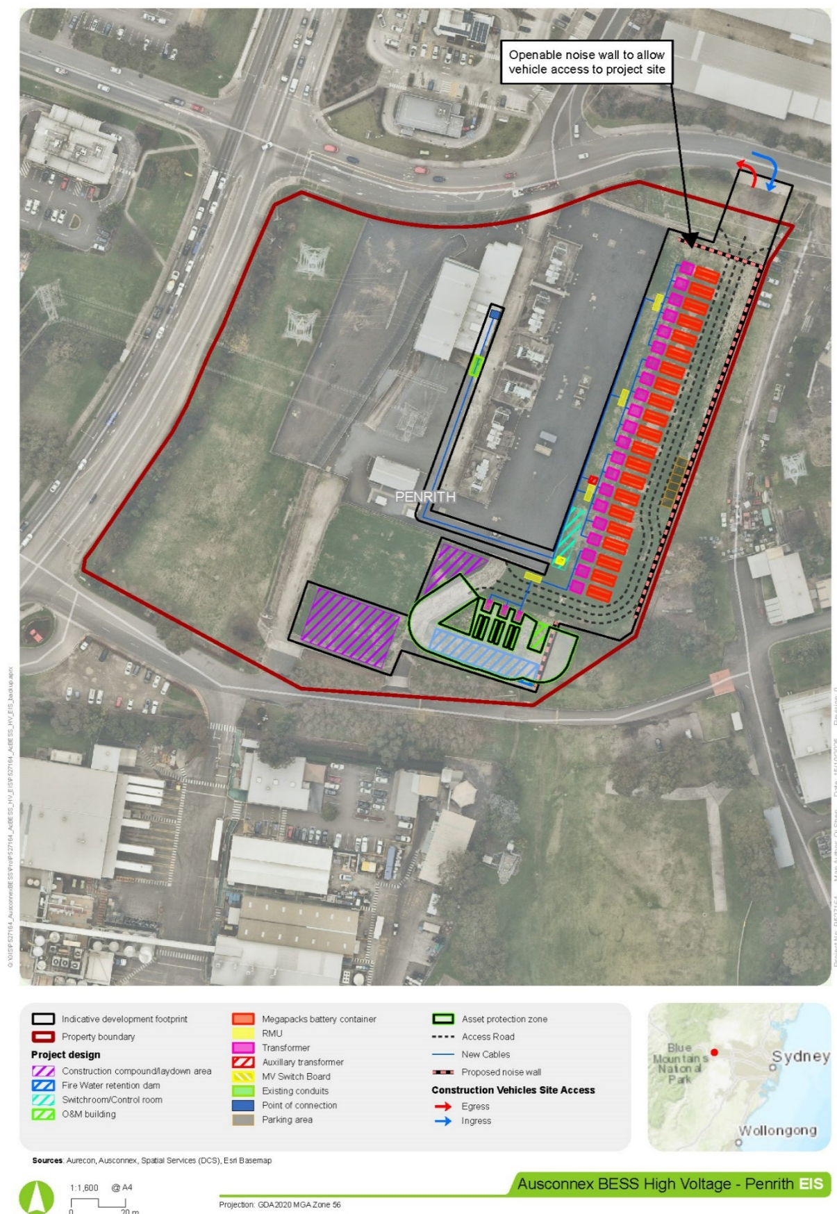
Figure 1-2: Penrith HV BESS Project layout
