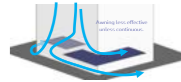
Figure 9: Schematic flow pattern around building with awnings
