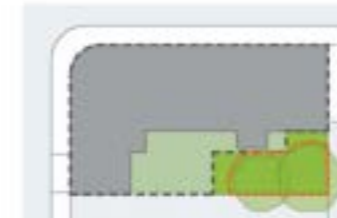
Figure 4O.5 Where trees are retained, tree protection zones need to be established during construction to protect the canopy and roots.
