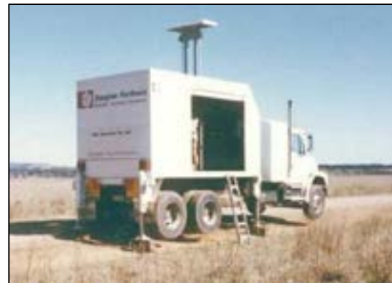
Figure 2: Purpose built CPT rig
