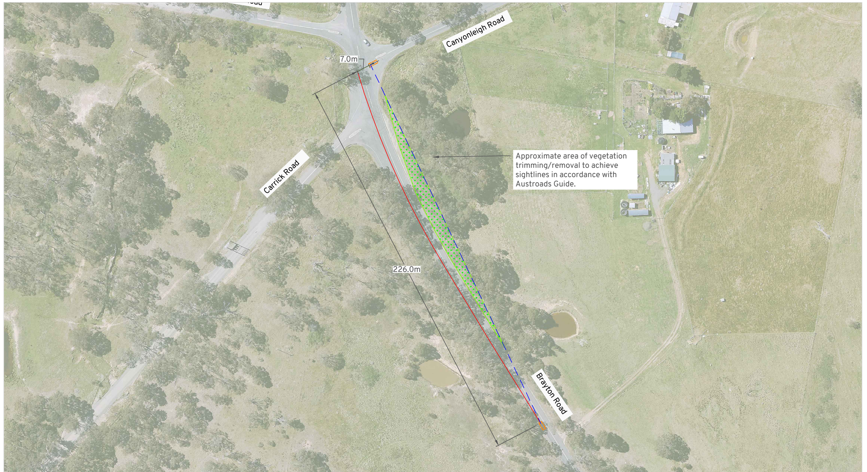
Brayton Road/Canyonleigh Road Intersection - Sight Distance to South
