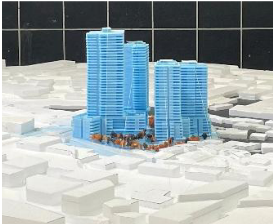
Figure 6: Close up view from the west of the 1:400 scaled model (with proposed landscaping) in the wind tunnel.
