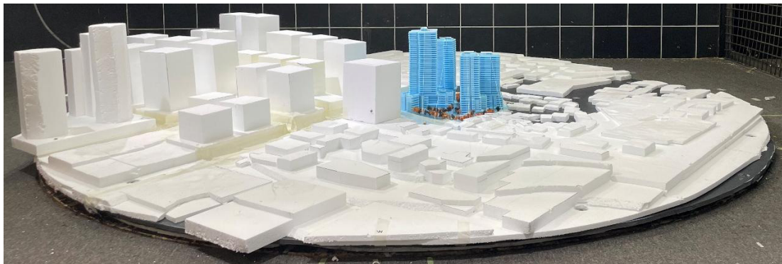
Figure 19: Overall view of the proposed development model in the wind tunnel (future scenario with proposed landscaping).
