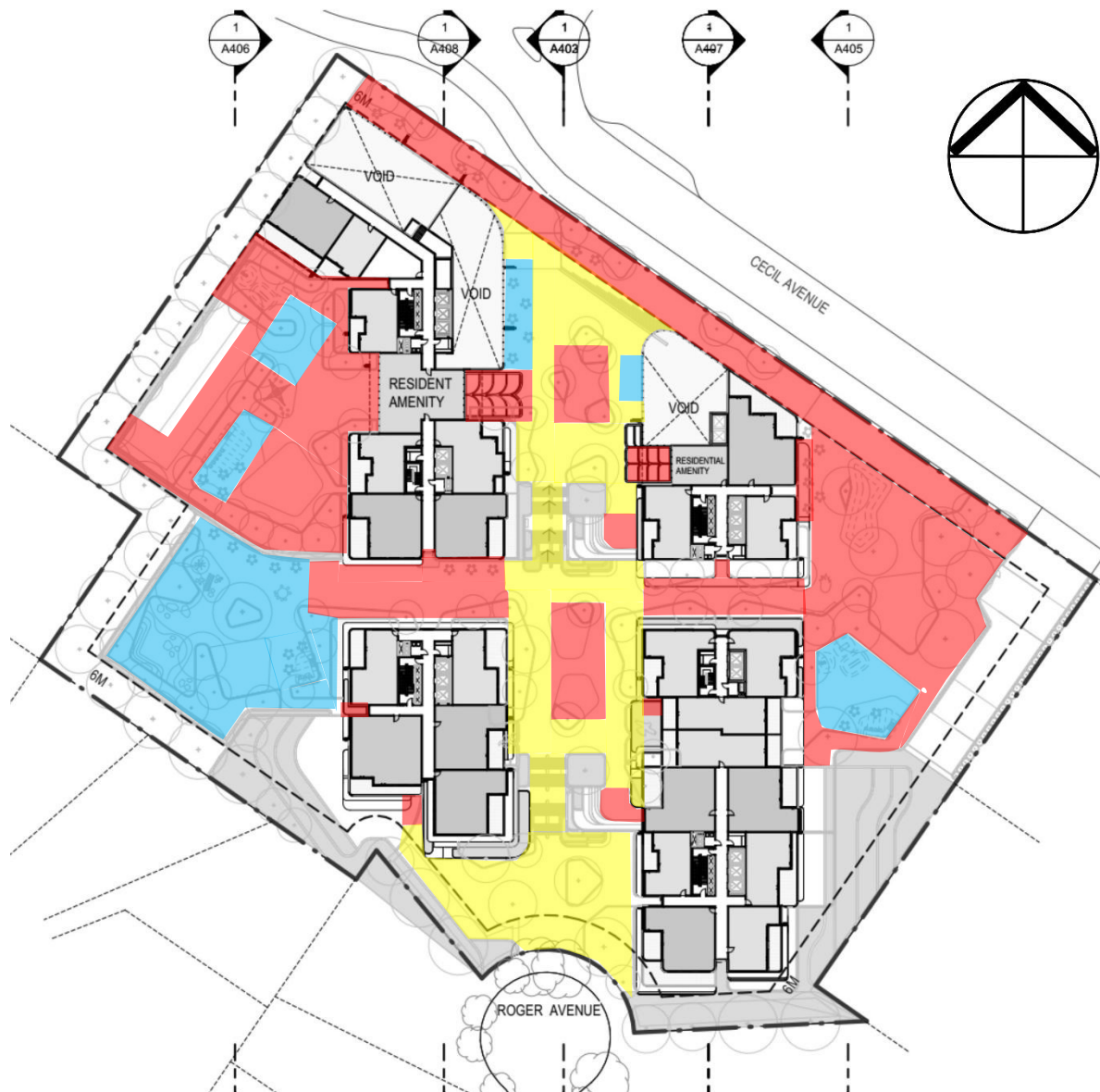
Figure 10: Ground floor plan within the development with recommended wind criteria overlaid.
