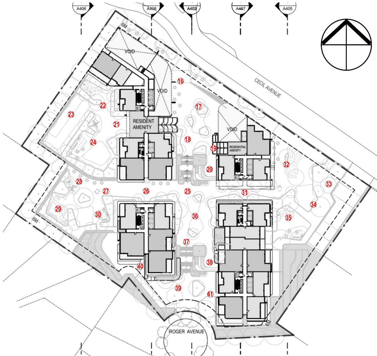
Figure 15: Sensor numbers and locations on ground level within project development.
