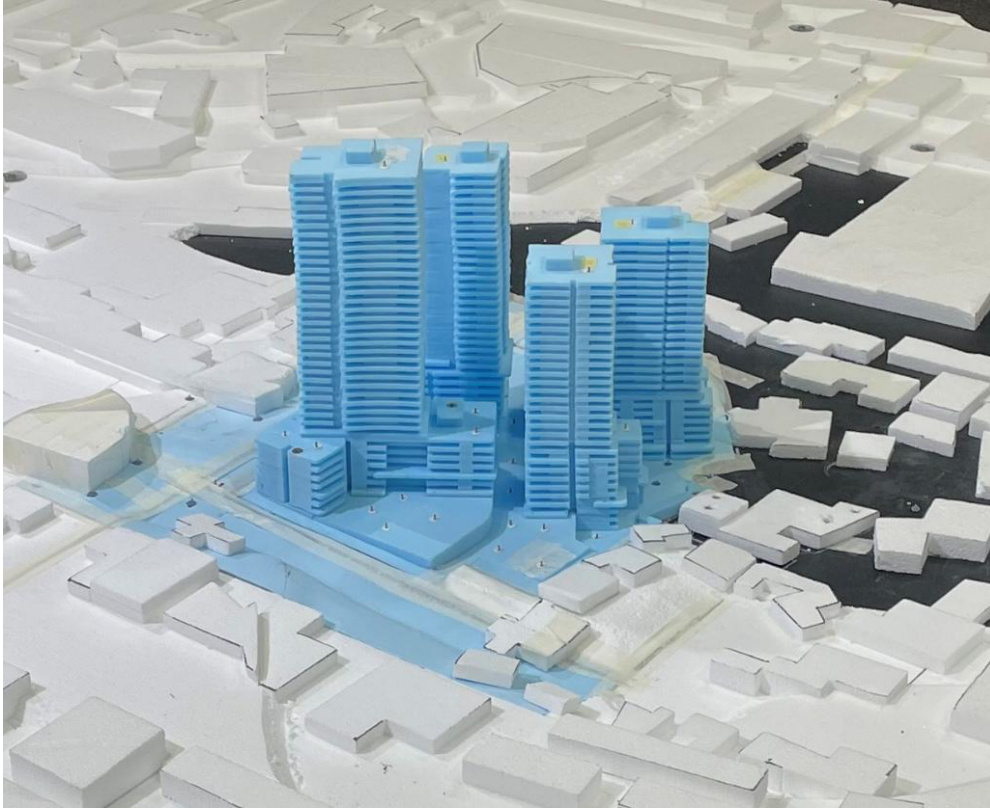
Figure 5: Overall view from west of the 1:400 scale model (without proposed landscaping) in the wind tunnel.
