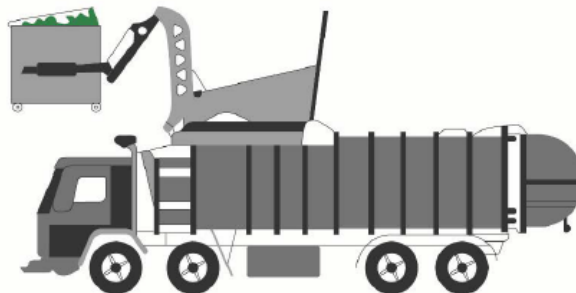
Front-lift-loading waste collection vehicle
