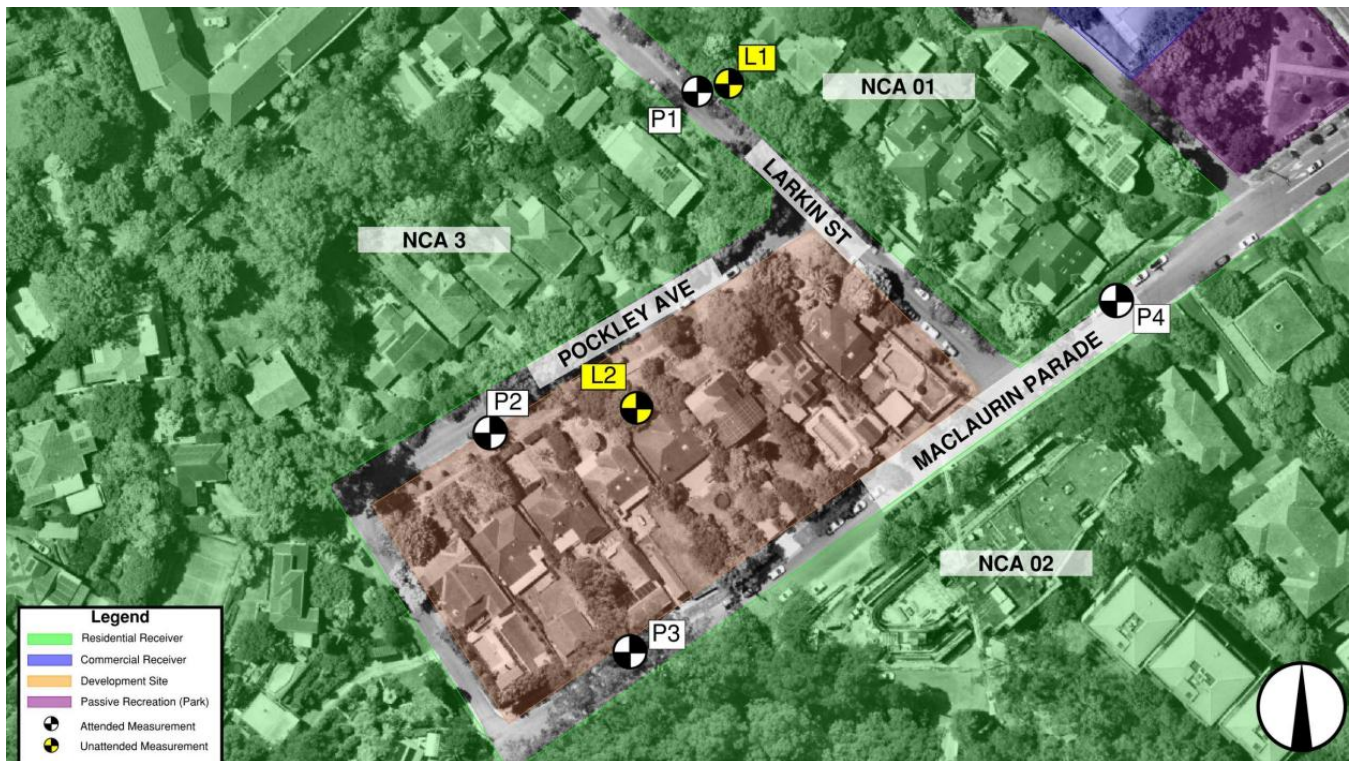
Figure 34 Overview of site and measurement locations identifying NCAs (Stantec)
