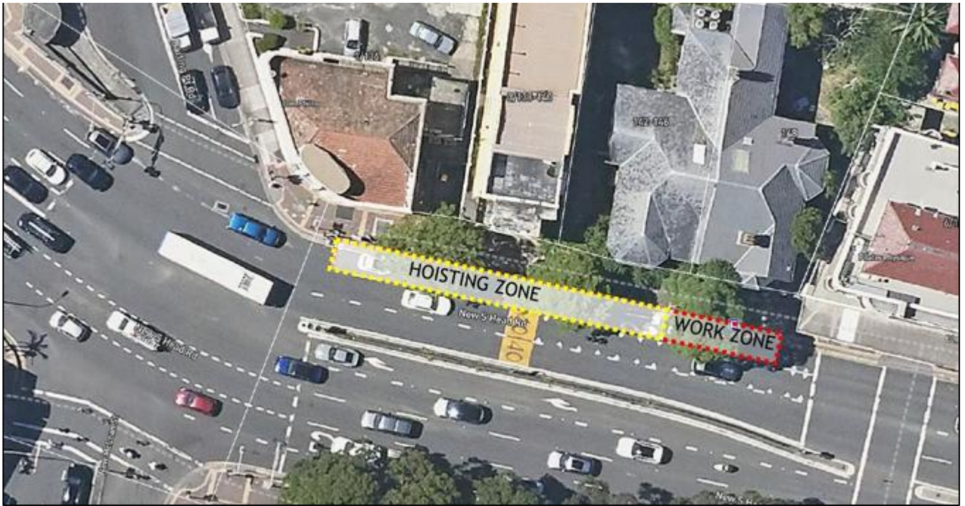
Figure 3 | Location of hoisting and works zone on New South Head Road (Source: Modification Application)
