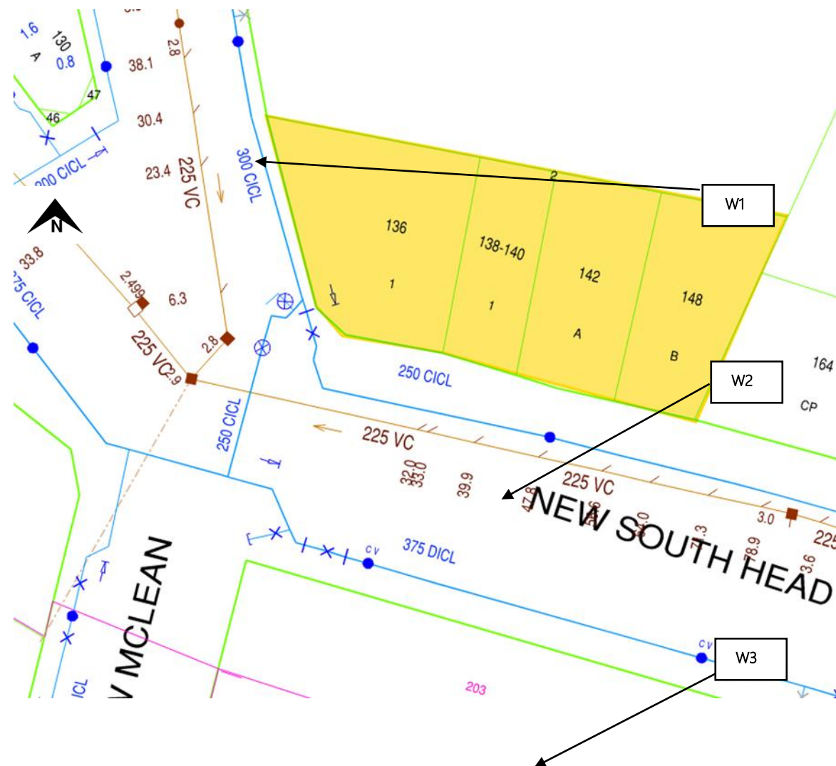
Figure 3: Authority Water Infrastructure
