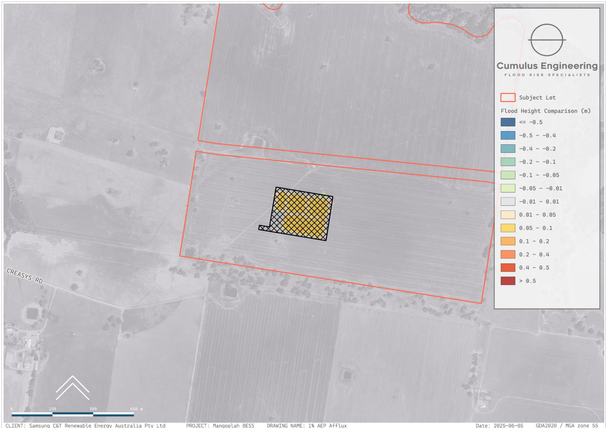
FIGURE 4-5 1% AEP AFFLUX Mangoplah Battery Energy Storage System - Flood Impact Assessment | NGH Consulting & Samsung C&T Renewable Energy Australia Pty Ltd
