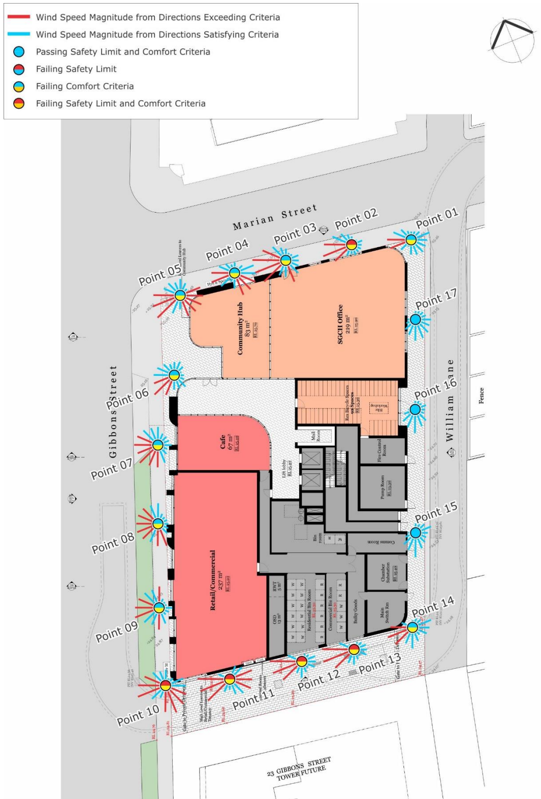
Figure 6a: Wind Tunnel Results – Ground Floor (results shown without treatments applied)
