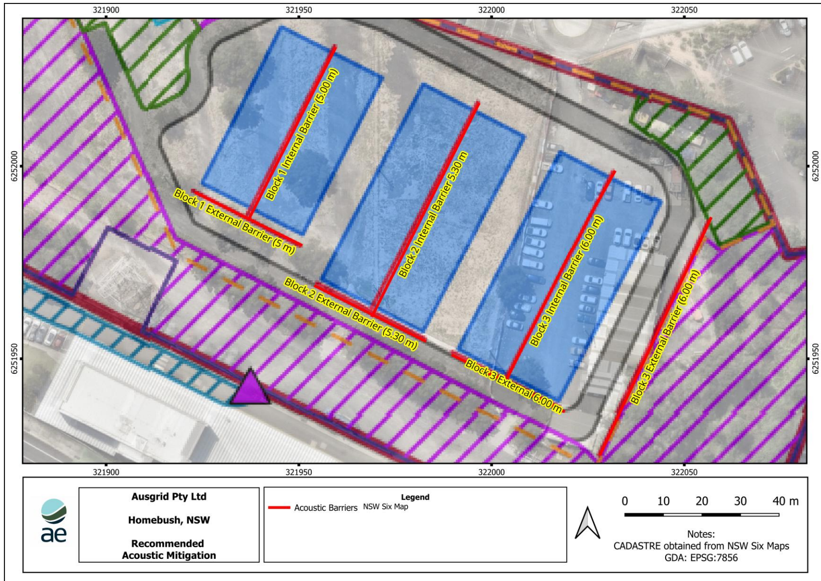
Figure 6: Noise Barrier Locations
