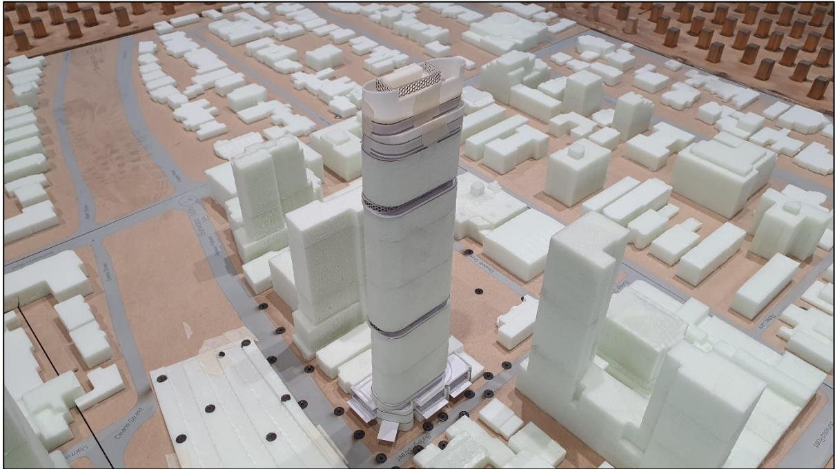
Figure 3 – View from the Northwest of the 1/400 scale Proposed Configuration model of the 2-4 Burleigh Street and 20-24 Railway Parade Development in the wind tunnel.
