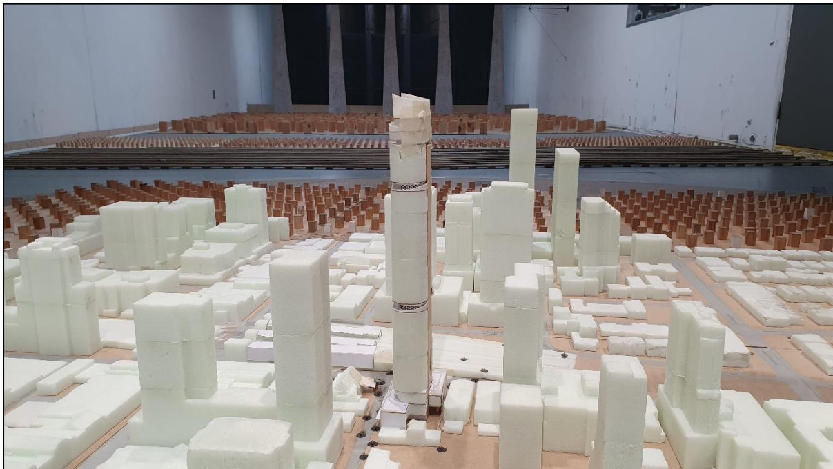
Figure 4 – View from the South of the 1/400 scale Proposed Configuration model of the 2-4 Burleigh Street and 20-24 Railway Parade Development in the wind tunnel.
