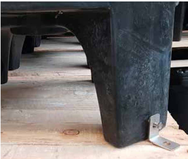
Figure 4 - Bolting the feet.
