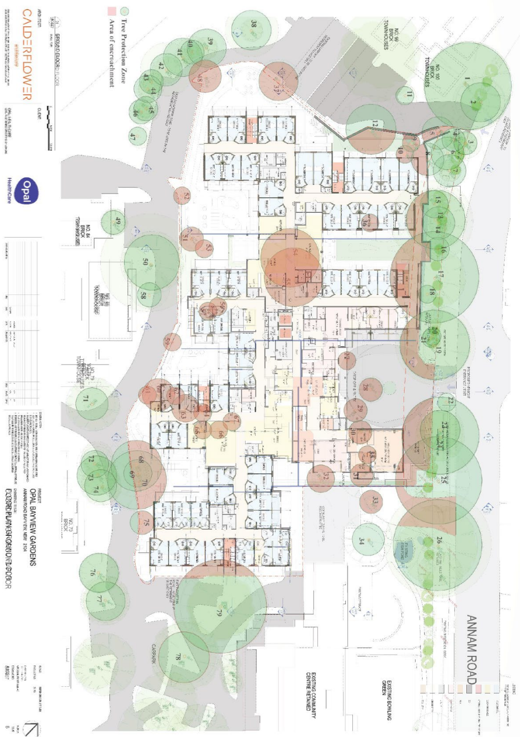
Figure 5: Showing the TPZ and area of encroachment
