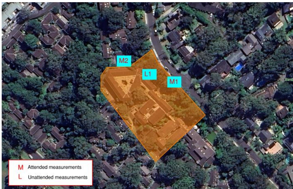
Figure 3: Long-term noise monitoring location (L1) and short-term noise monitoring location (M1).
