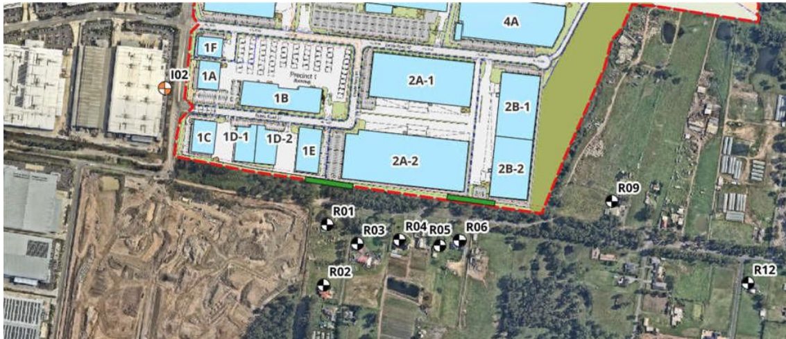
Figure 28: Location of permanent noise walls shown in green at southern boundary of Precinct 2 (Source: RWDI)
