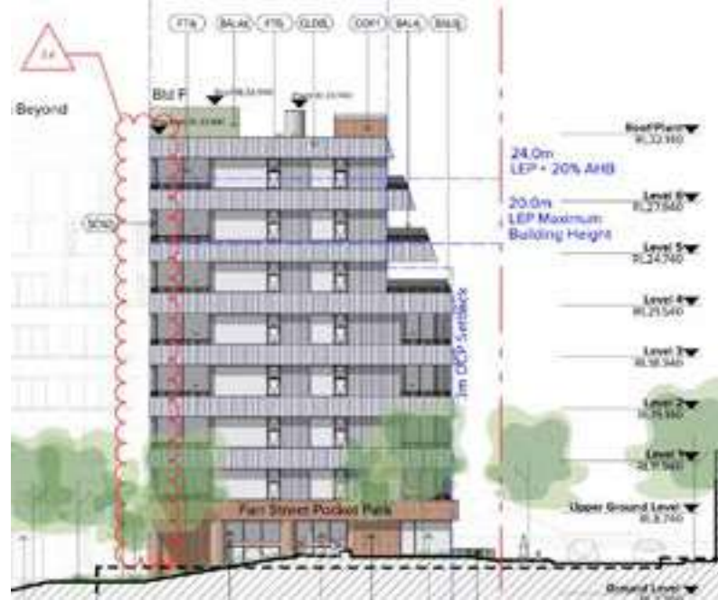
Approved SSDA - DA-220-301_ Warehouse Place North Elevation
