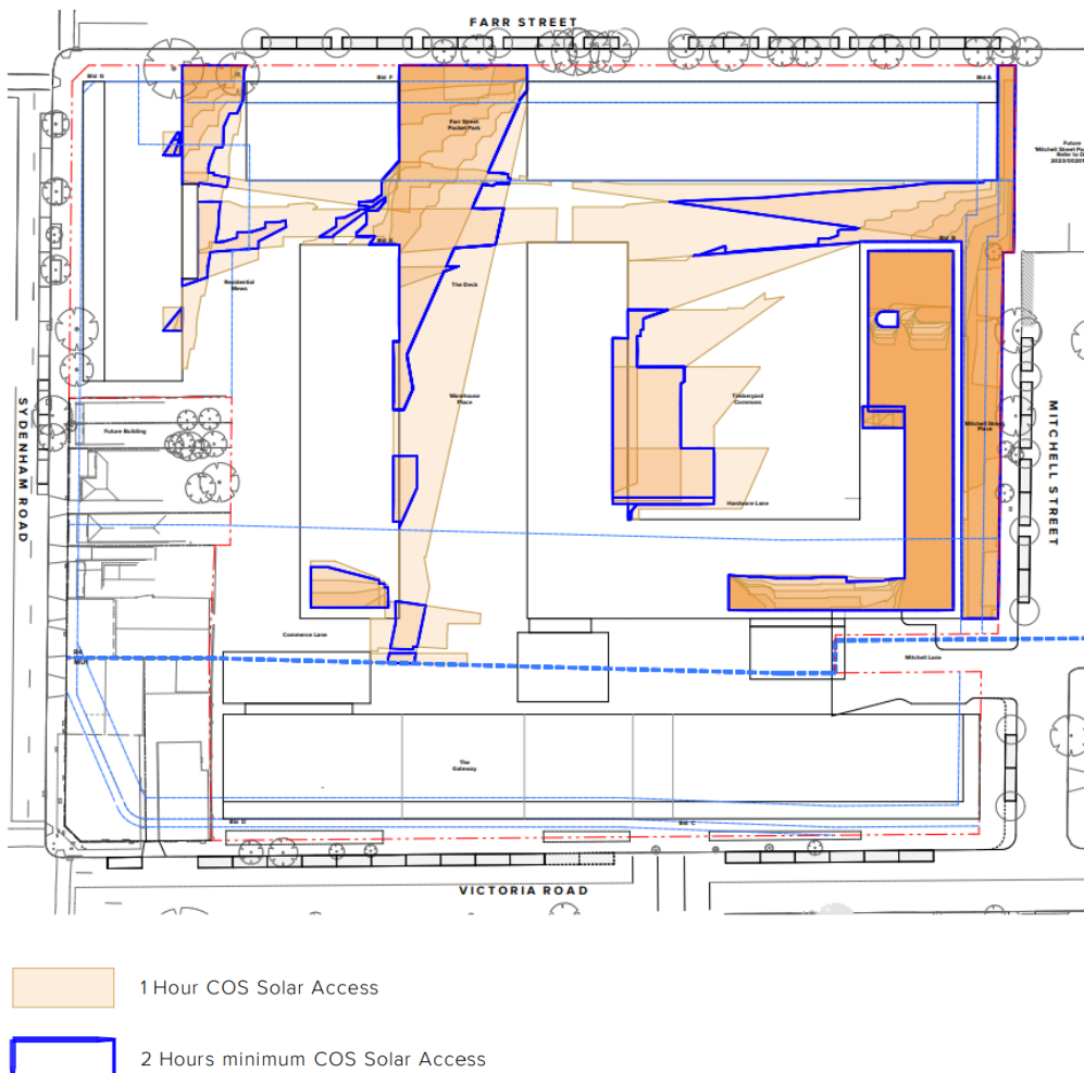
Figure 58 Solar amenity to common open spaces
