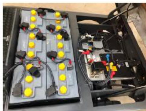
ST3000-AC tow tug complete with 6 x 250AH heavy duty batteries
