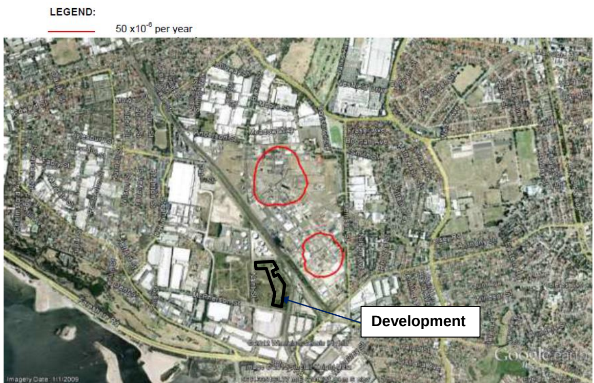
Figure 5.4: Property damage – overpressure 14 kPa (BIP QRA report, Ref. 7)
