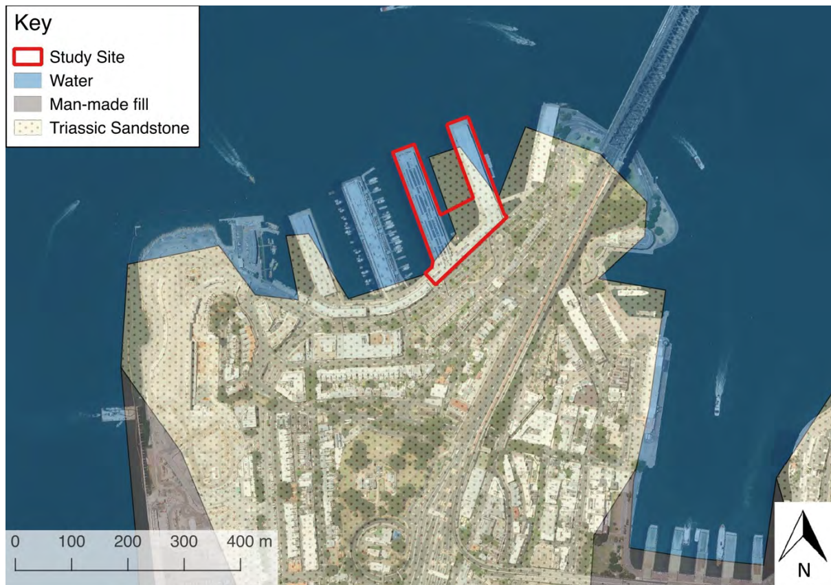
Figure 4 Map of the local underlying geology of the study site. (Source: NSW Geological Survey with CRM additions)
