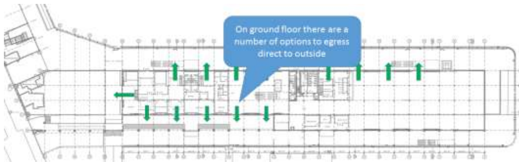
Figure 14: Pier 2/3 Ground Floor exits
