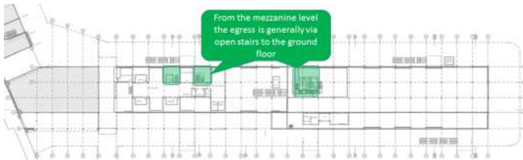
Figure 15: Pier 2/3 Mezzanine level egress
