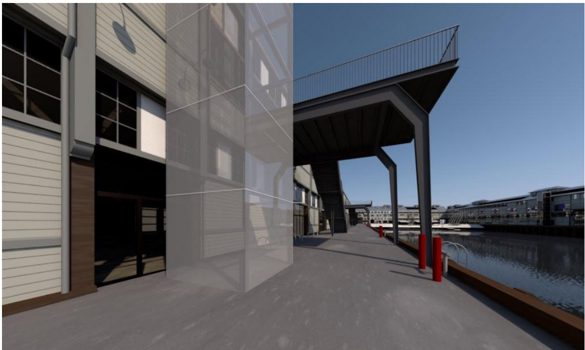
Figure 77 - 78: 3D representation of the proposed new external lifts, rendering by TGZ. 25
