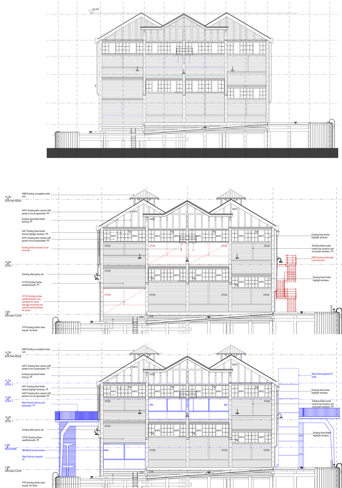
Figure 84: Pier 2/3 North Elevation Existing - Demolition - Proposal. Demolitions in red and Proposal in blue. Drawing from TZG Architects.
