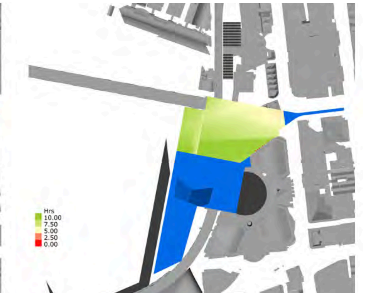
Fig. 67. Solar access analysis of the new park on 4 April
