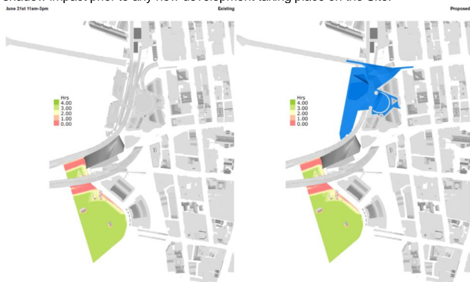
Figure 38 – Overshadowing impact of the proposed envelope on Tumbalong Green (site area shown in blue)
