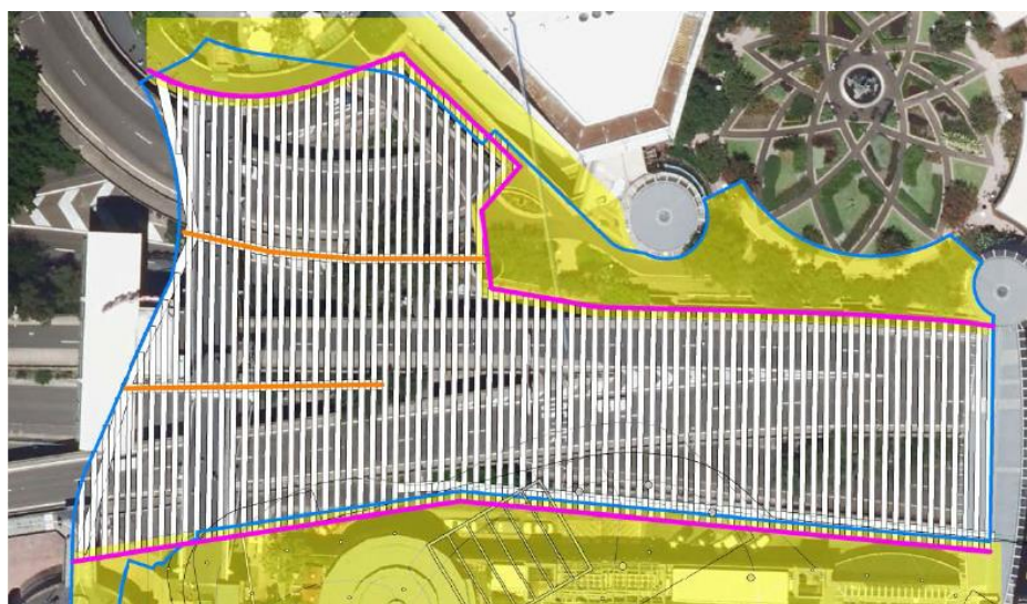
Source: Figure 34 – Overbridge beam layout Source: Enstruct
