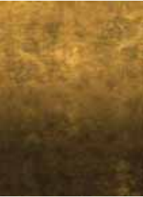
BR1 - Brass plate to counter fronts with gradually darkened patina. Top of brass counter to be natural/ off the mill brass colour, bottom to be pre-aged/ burnished brass colour
