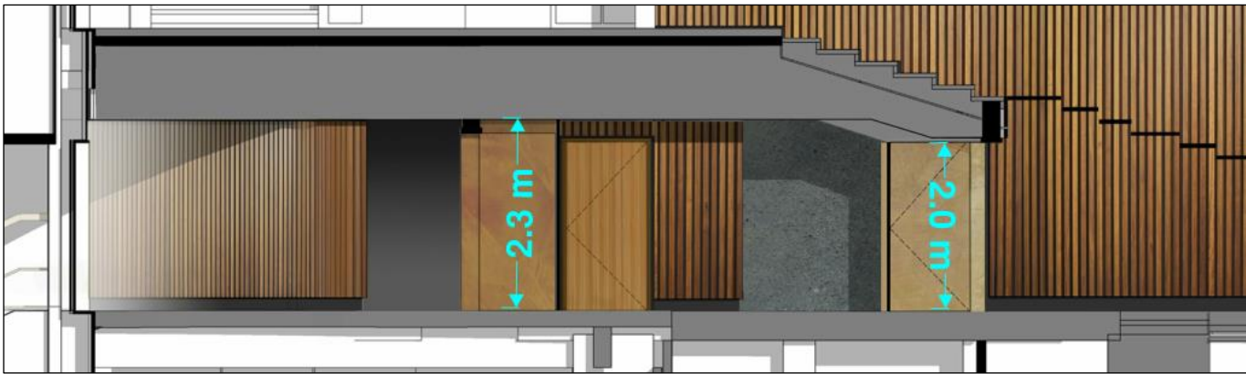
Level 3 Passageway Low Ceiling Height
