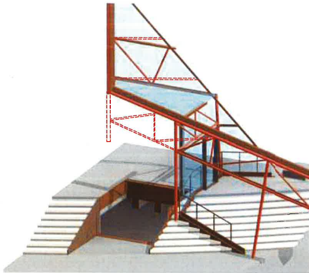
3D Image of Removed Steel Structure
