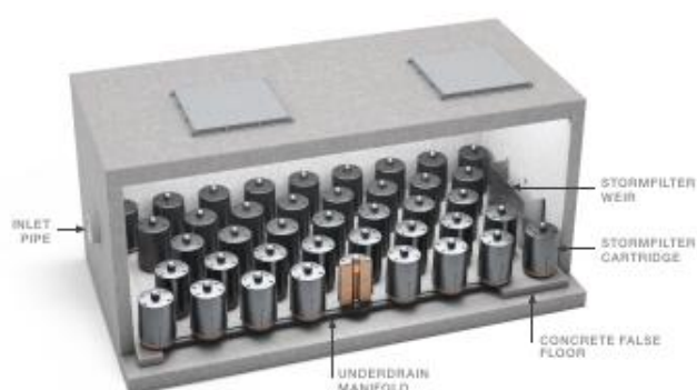
Figure 2: Example conceptual diagram of a StormFilter® system
