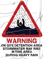
OSD WARNING SIGN N.T.S. SUGGESTED SIZE 600mm x 450mm TO BE PROVIDED ADJACENT TO OSD TANKS / OSD BASINS IN SUITABLE AREA T.B.C ON SITE
