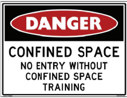
CONFINED SPACE SIGN N.T.S. SUGGESTED SIZE 300mm x 450mm TO BE PROVIDED ADJACENT TO OSD TANKS / DCP OUTLET PITS IN SUITABLE AREA T.B.C ON SITE
