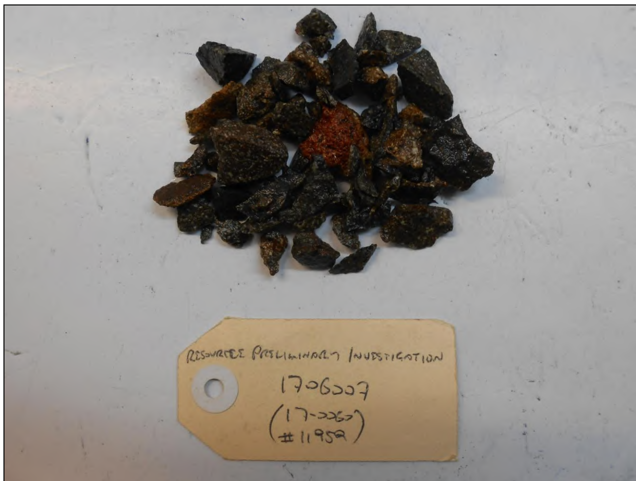
Plate 1: Photograph of supplied crushed aggregate sample.
