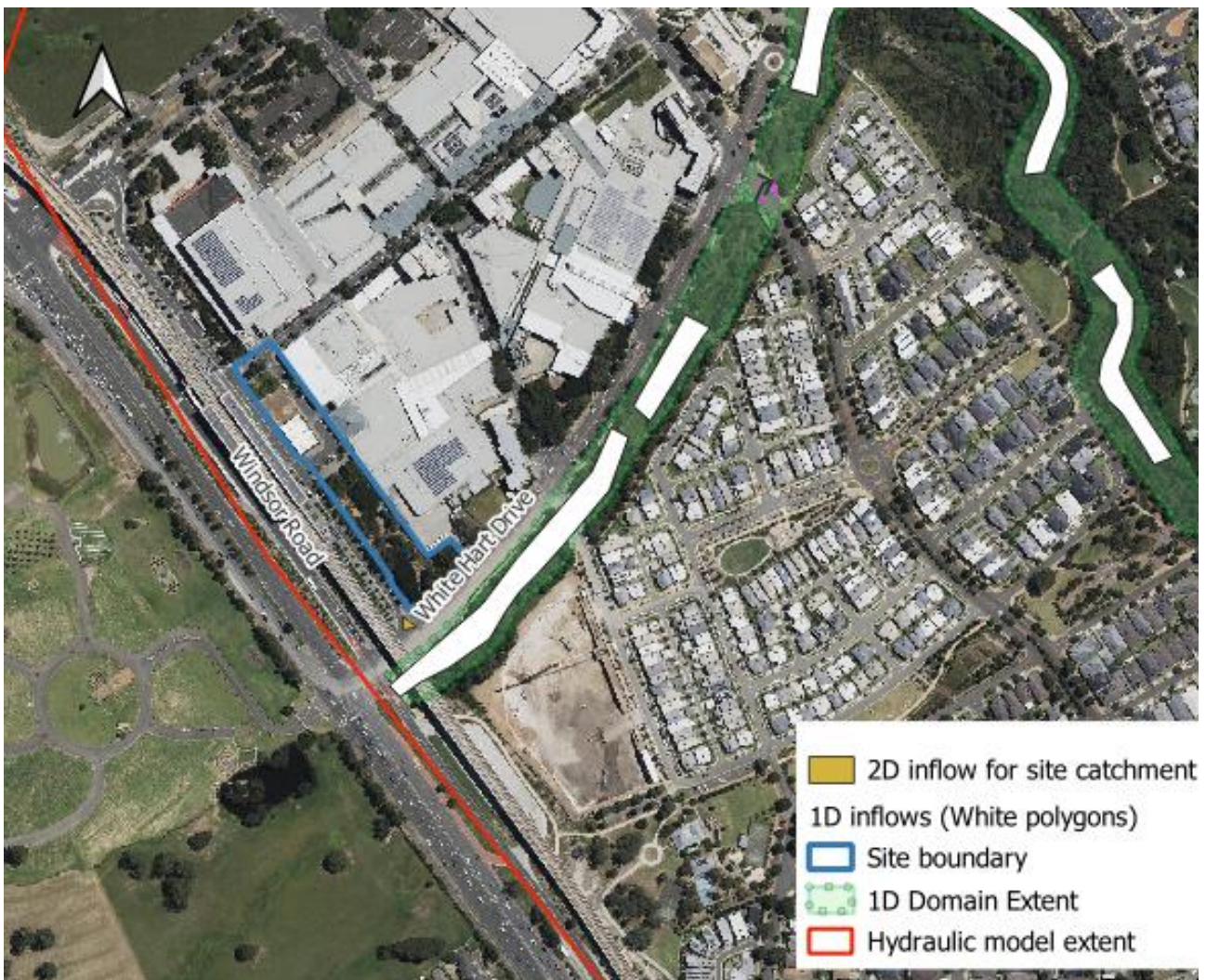
Figure 3-5 Inflow Boundary Conditions near the Site in the Updated TUFLOW Model
