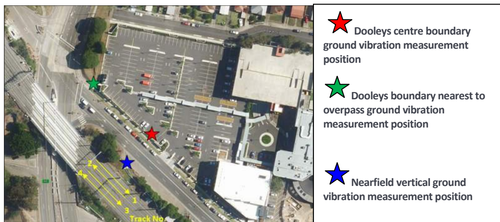
Figure 14: Vibration measurement positions
