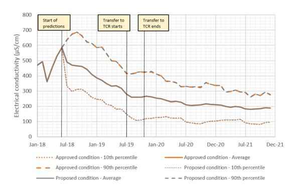
Figure 3.8 Approved condition vs proposed condition electrical conductivity on Coxs River directly upstream of Lake Burragorang
