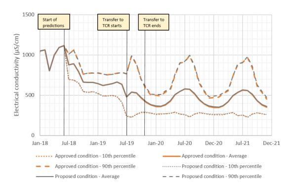
Figure 3.4 Approved condition vs proposed condition electrical conductivity on Coxs River at the confluence with Pipers Flat Creek
