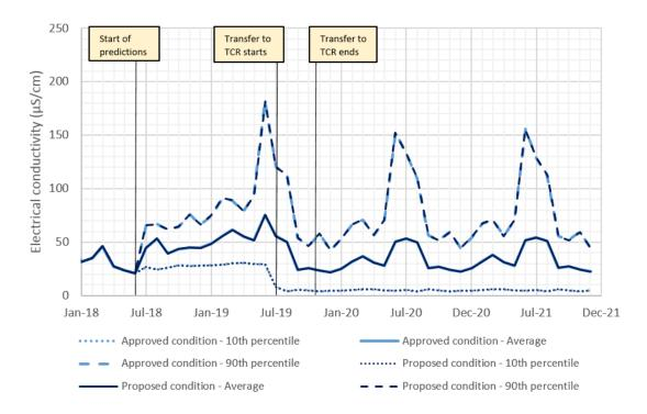
Figure 3.5 Approved condition vs proposed condition flows on Coxs River directly upstream of Lake Wallace
