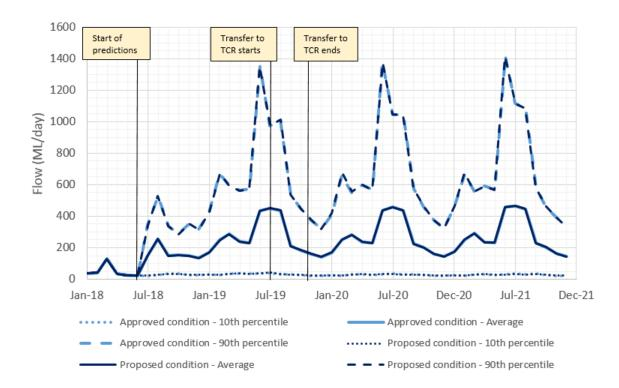
Figure 5-6 Approved condition vs proposed condition flows on Coxs River directly upstream of Lake Burragorang
