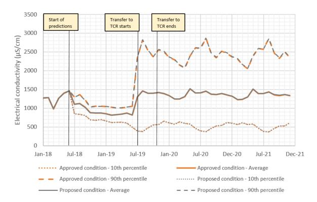
Figure 5-5 Approved condition vs proposed condition electrical conductivity on Coxs River directly upstream of Lake Wallace
