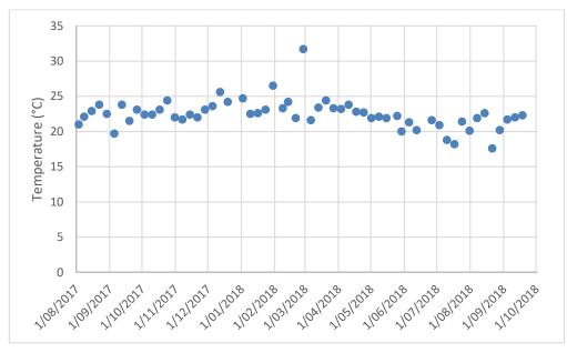
Figure 5-1 Temperature of mine water, August 2017 – September 2018
