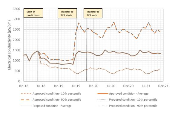
Figure 3.6 Approved condition vs proposed condition electrical conductivity on Coxs River directly upstream of Lake Wallace
