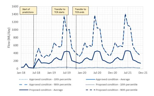
Figure 3.7 Approved condition vs proposed condition flows on Coxs River directly upstream of Lake Burragorang
