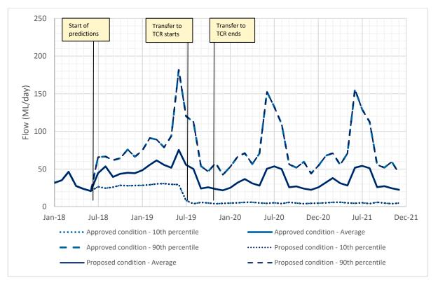
Figure 5-4 Approved condition vs proposed condition flows on Coxs River directly upstream of Lake Wallace
