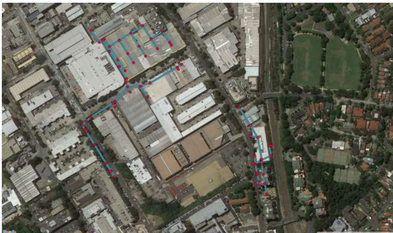
Figure 2 – Existing Underground Drainage System within the Catchment
