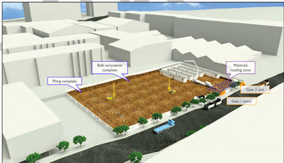
Figure 3: Site Establishment and demolition
