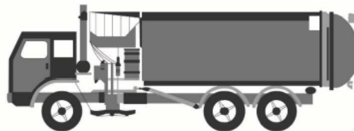
Side-loading waste collection vehicle
