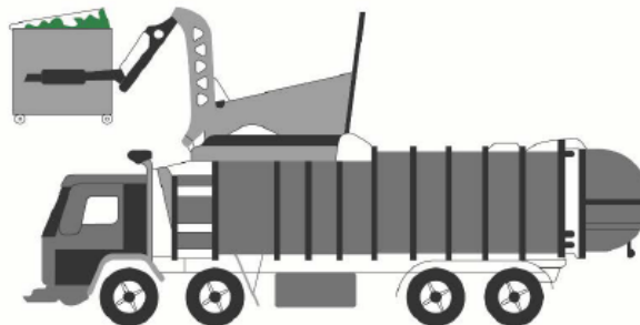
Front-lift-loading waste collection vehicle
