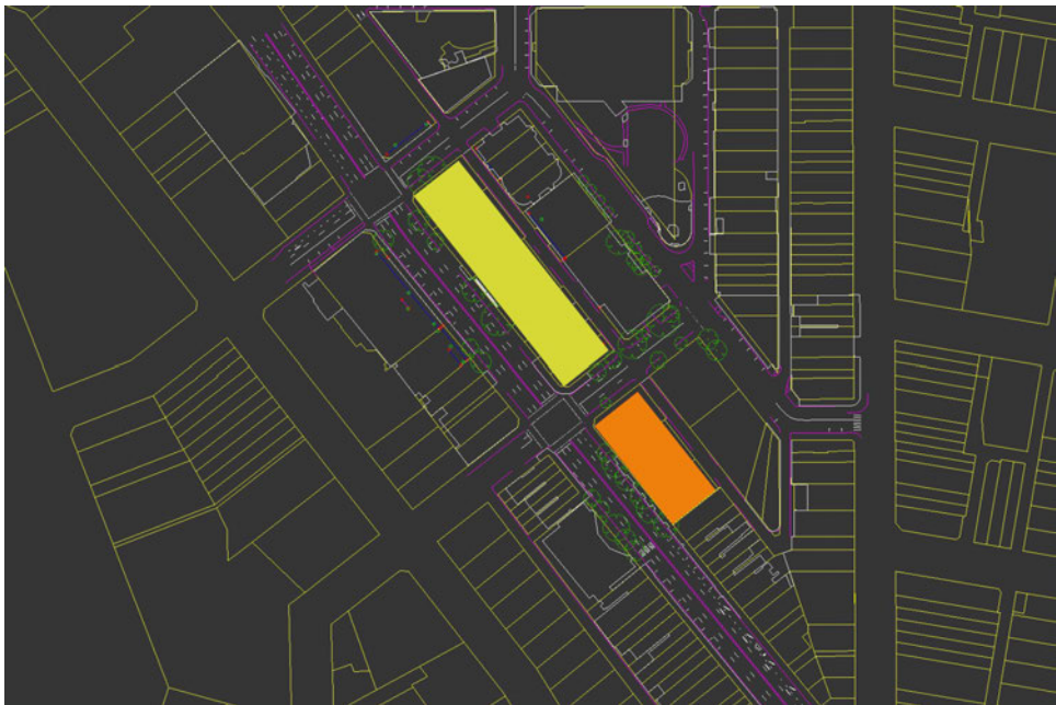
Image showing survey drawing supplied at MGA 56 GDA2020 and 3D model of the proposed amending building envelope aligned to the site boundary
