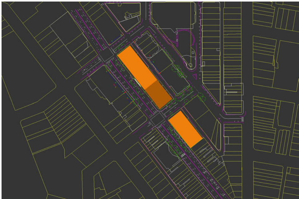
Image showing survey drawing supplied at MGA 56 GDA2020 and 3D model of the approved building envelope aligned to the site boundary
